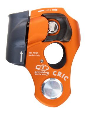
Multifunctional rope clamp with integrated pulley for mountaineering, rope access work and rescue. Robust, practical and intuitive, it has four different modes of operation: ascender, pulley, rope clamp/pulley or progress-capture hauling pulley.
